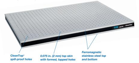
Another in a long line of TMC innovations, our 75 Series Breadboards minimize both weight and cost. A patented manufacturing technique allows us to form countersunk, tapped holes in a thin top skin of stainless steel. The holes are not drilled or punched, but fabricated in a way that effectively "thickens" the skin in a small ring around the threads. No inserts are used and the tapped holes are three threads deep.
